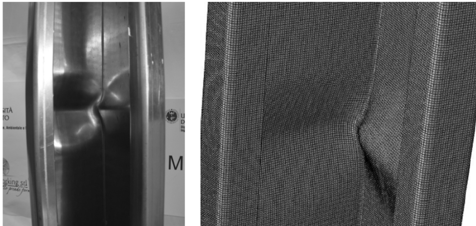
Fig. 5. Experimental and numerical collapse of the specimen under pure compression
