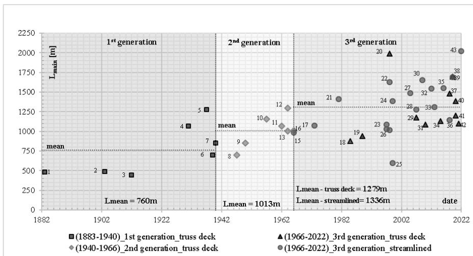
Fig. 9. Growing main span ( $L_{main}$ ) from 1883 to 2022
