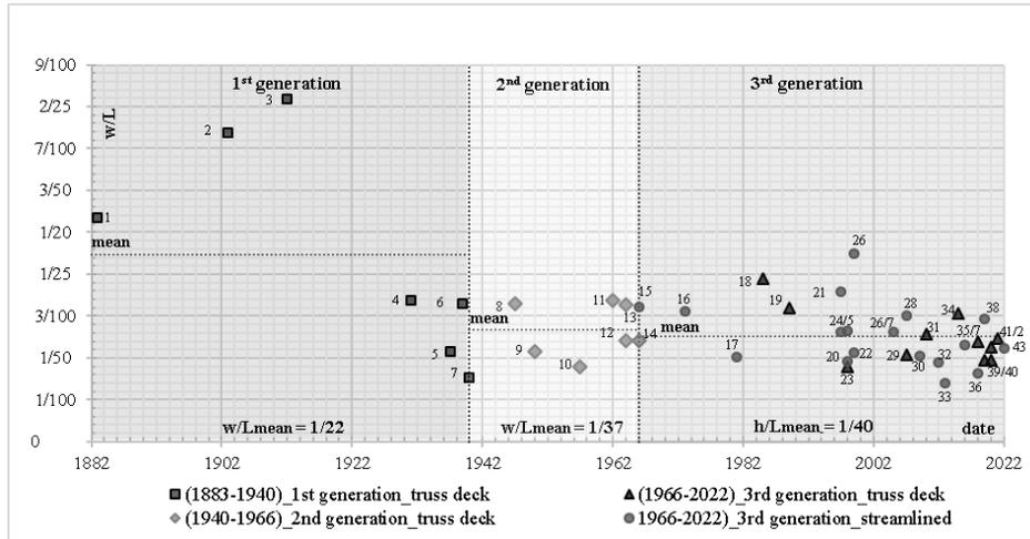
**Fig. 11.** Deck torsional stiffness ( $w/L$ ) from 1883 to 2022
