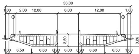
Fig. 12. Suspension bridge historical evolution: deck cross section details
