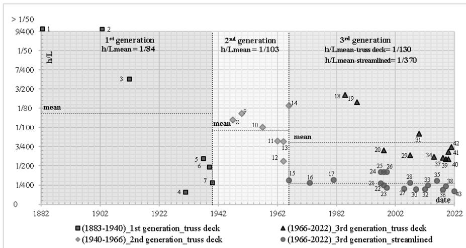
Fig 10. Deck slenderness ( $h/L$ ) from 1883 to 2022
