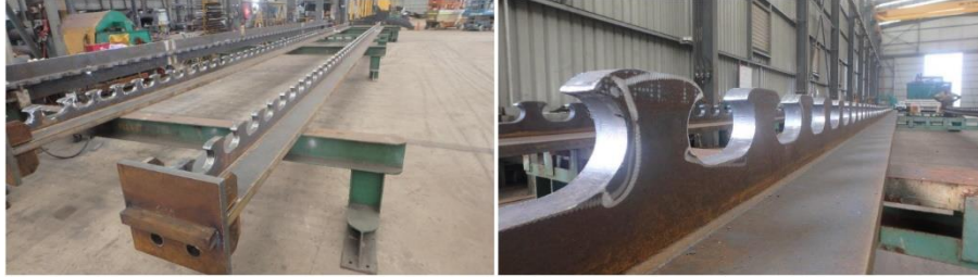
Fig. 3. Example of built-up cross sections type A used for 0207A bridge in Western Australia [6].
