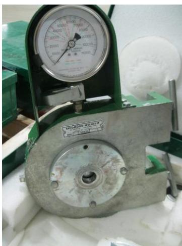
Figura C11.2 - Bolt Tension Calibrator (Shidmore-Wilhelm)
